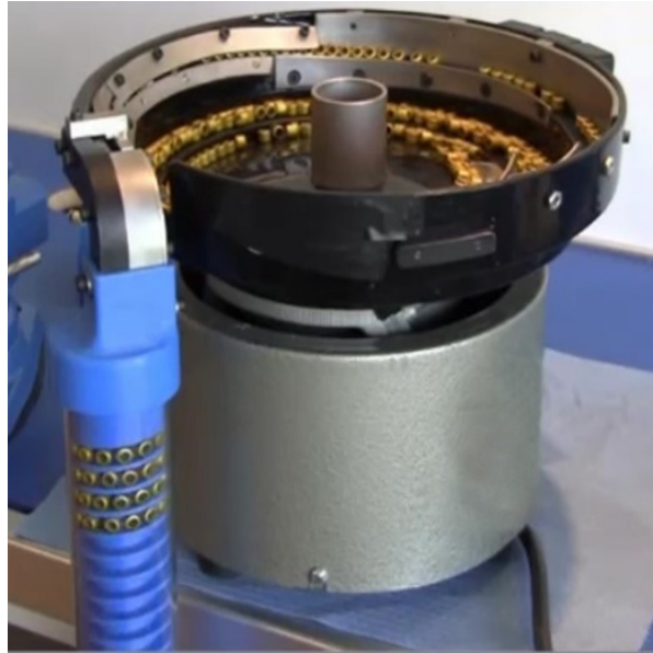
Collar Feeder Bowl Feeds collars in Cartridge Contact Gage Bilt for more information. (Sold Separately)
