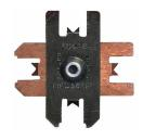
Gage Bilt also supplies pin & collar swage inspection gages to certify correct swage installation
